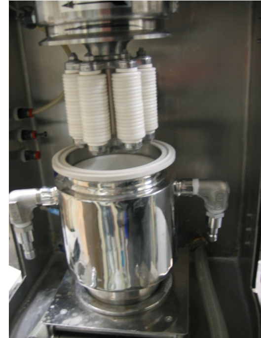
Nara Machinery Co.'s MIC 0 zirconia ring/zirconia-lined wet milling machine from the Riman laboratory.
