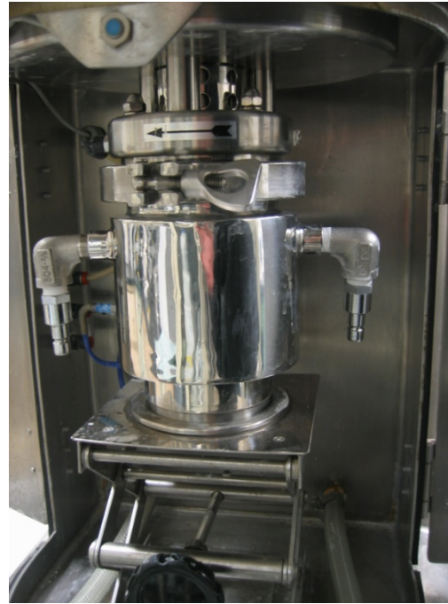
Nara Machinery Co.'s MIC 0 zirconia ring/zirconia-lined wet milling machine from the Riman laboratory.
